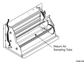
Fig. 20 - Return Air Sampling Tube Location
